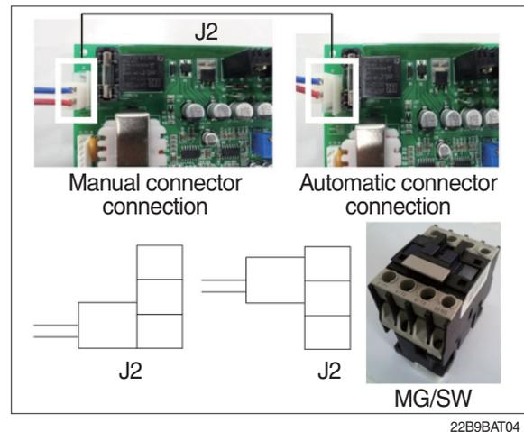
(4) **Checking charging voltage soft start function (Refer to the monitor)**
