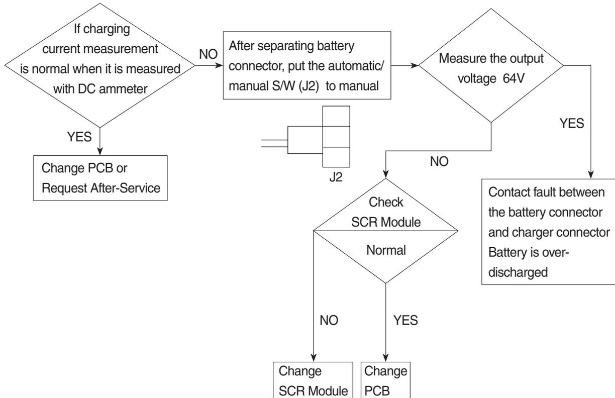
⑥ Charger has no response even if the battery connector is connected.
