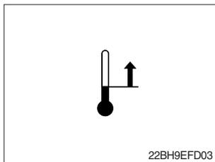
This LED lights when the controller or motor temperature is high.
