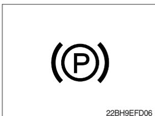
(1) This LED lights when the parking brake is activated.
